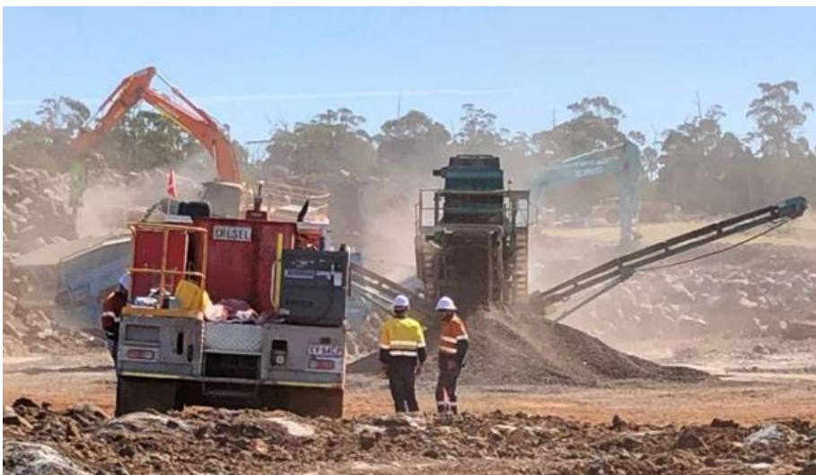
Plate 23: Site Quarry Processed for Pavement Materials, Dundonnell Windfarm, Victoria
