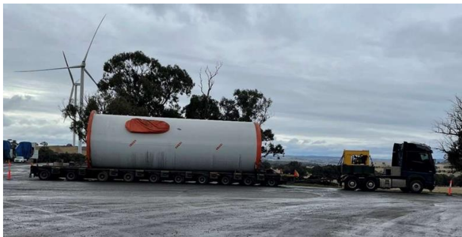
Plate 14: Heavy Load Platform: used for gearboxes, nacelle, shorter tower segments, main power transformers
