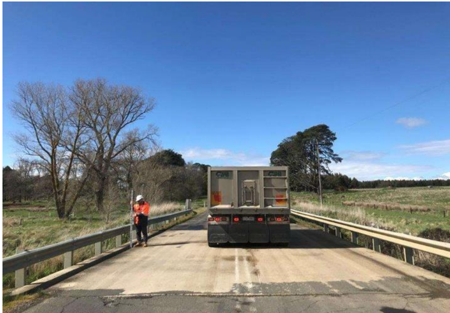
Plate 17: Load Testing of 1940's Bridge – Lal Lal Windfarm, Victoria
