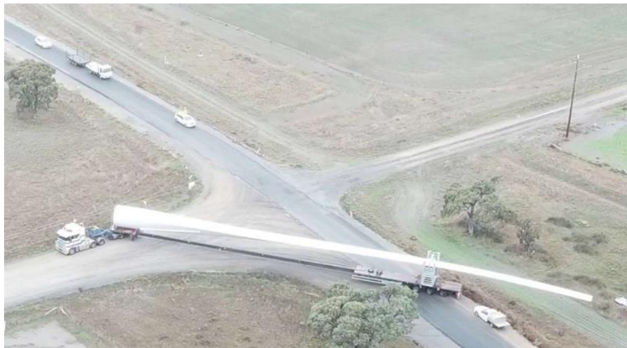
Plate 15: Telescopic Trailers for blade deliveries
