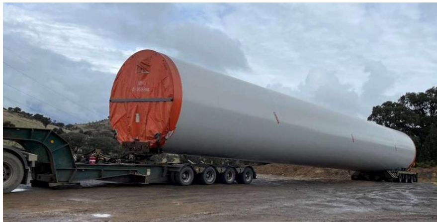
Plate 13: Beam Trailer: used for long tower segments, switchroom
